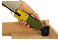
wood, PC cards, plastics, plaster of Paris and many other materials. The segment cut facilitates exact cutting right into corners.
