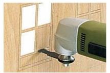
For precision square excavations, HSS immersion saw blades are available with an 8 and 14mm width of cut.
